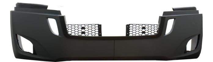
Designed to fit the New Cascadia 116/126 applications. The Alliance composite bumpers are a light weight, cost-effective alternative to OEM composite bumpers. Built with premium materials to ensure product quality and durability without premium pricing. Two-piece design, lighter weight and lower cost than OEM composite bumpers.
