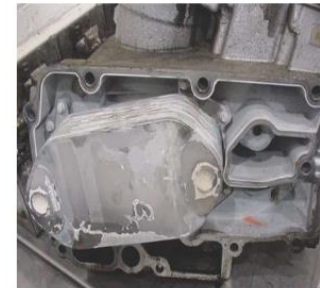
Aluminum Corrosion with NOAT
