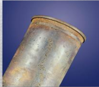
Or Wet Sleeve Cylinder Liner Pitting
